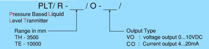
ex:Pressure Based Level Transmitter for range of 3.5mtrs with 0....10 VDC PLT / R - $\overline{TH}$  / O - $\overline{VO}$  /
