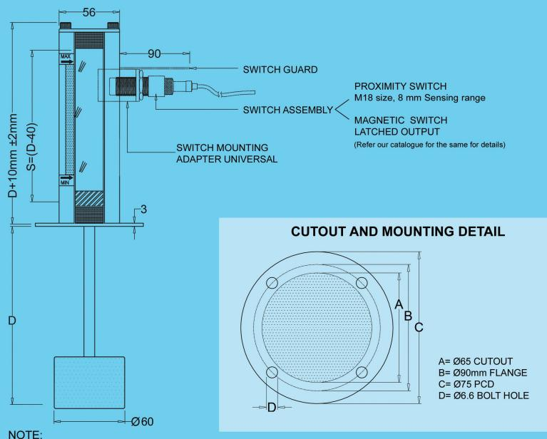
Min, Max, Green Band Stickers are Supplied Loose. To be fixed at site. For selection of Switch Assembly refer Magnetic Proximity switch Catalogue.
